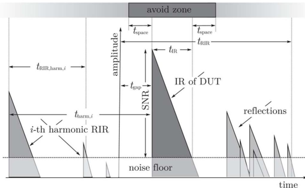
**Figure 4 – Temporal structure of an impulse response measured with an exponential sweep.**
