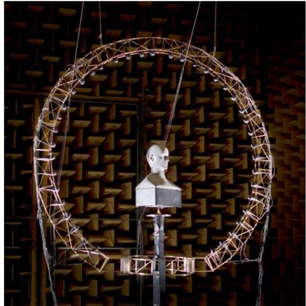
**Figure 5 – Photo of the HRTF measurement set-up while measuring the HRTFs of a dummy head.**
